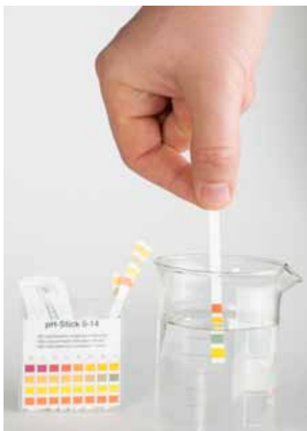
Right: A litmus strip is one of the fastest and economical ways of determining whether or not water is acidic; Below: Water sampling procedure for microbiological analysis
